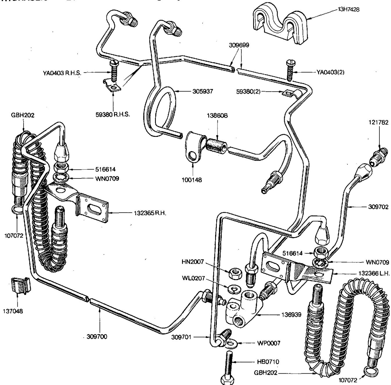
**HYDRAULIC PIPES – Front L.H.S. – Single System**
